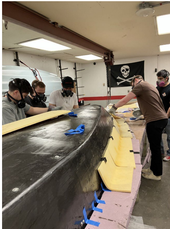
Figure 6: Forming Gurit Corecell Foam Mold to the Hull
