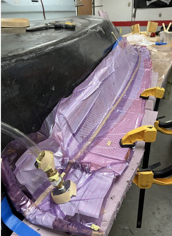
Figure 7: Fiberglass Layup to Form Mold for Carbon Fiber
