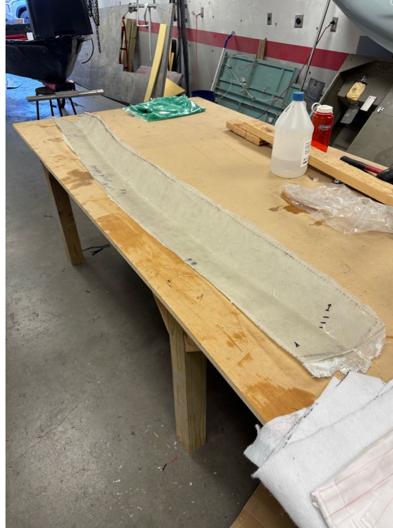
Figure 8: Final Fiberglass Mold to Use for Carbon Fiber Layup
