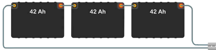
Figure 6: The battery layout for the 2019 year's endurance mode consists of three 42 Ah batteries in series for a total of 42 Ah.
