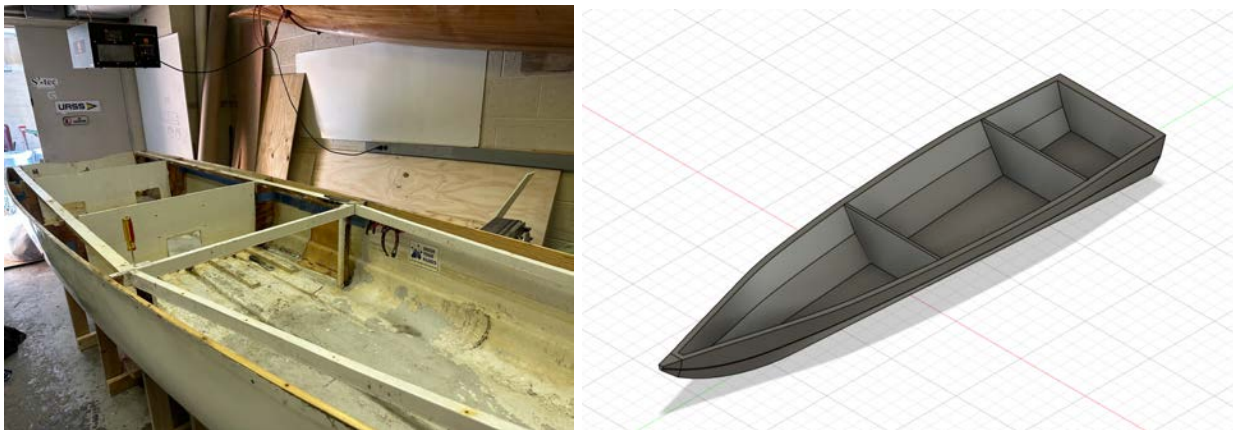
Figure 26: Left: Closeup of the transom, which had rotted out and needed replacement. Right: CAD model of the planned hull reinforcements, which would replace the benches.
