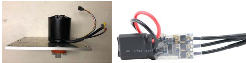
Figure 7: Left: The Alien Power Systems 6374S motor used by the 2019 team for Endurance mode. Right: The VESC 4 motor controller is used in Endurance with the motor.
