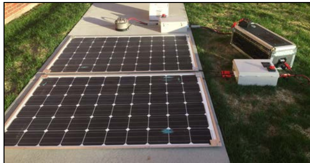
Figure 23: An example of our solar testing in the field: Both panels connected to the system at dusk and in partial shade. Our team plans to perform a number of these tests at different light intensities and weather conditions.
