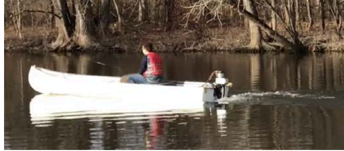
Figure 12: 2019: The boat was in the water during a testing session in December, during which we tested the drivetrain's efficiency at low speeds.
