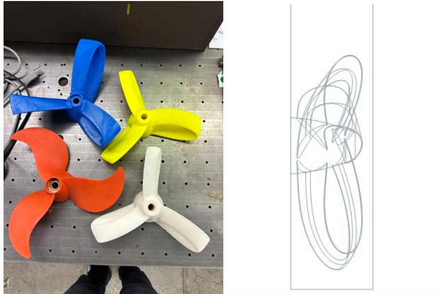
3D printed models and Static wireframe view of rotating region geometry in NX.
