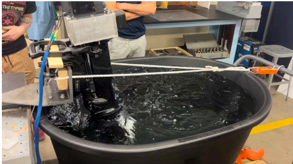
Figure 11: Inside the test room, a tub of water with the propeller is submerged. The motor stand has a force gauge meter strung around it to collect thrust.
