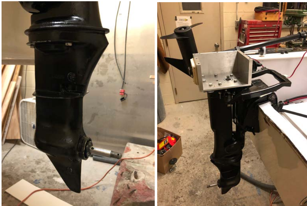
Left: The modified outboard lower unit, with the ventilation plate cut back to allow for larger propellers. Right: The outboard motor with a frame of the upper unit, mounted on the boat hull.
