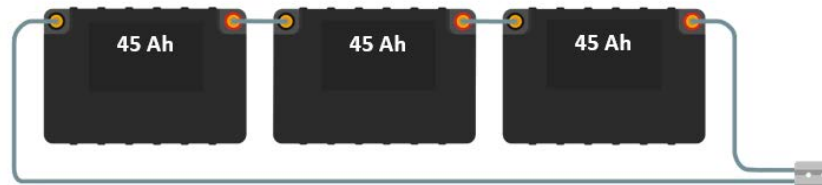
Figure 8: The 2024 battery layout consists of three 45 Ah batteries in series, for a total of 45 Ah at 36V.
