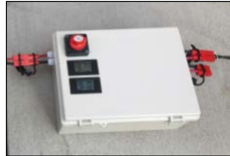
Figure 21: The previously completed solar charger module, with solar charger input/battery output cables, current monitoring LCDs, and an on/off switch.
