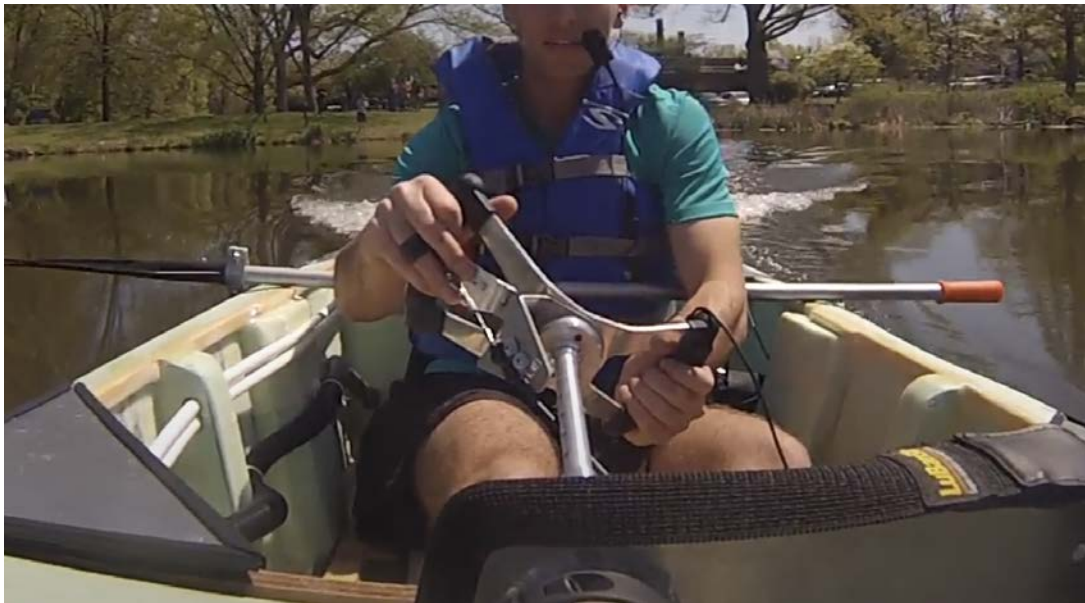
Fig. 7.6- Steering and throttle functionality in wet tests (microswitch not pictured)
