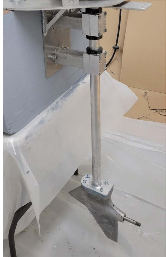
Fig. 6.6b- Endurance output shaft and lower unit, supported by standoffs
