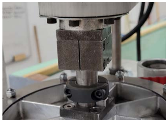
Fig 6.5- Double-sided shift dog on output shaft, engaged with sprint drive ratio
