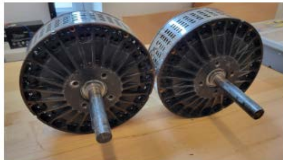
Fig. 6.3- Two Lynch LEM 200-D126 motors
