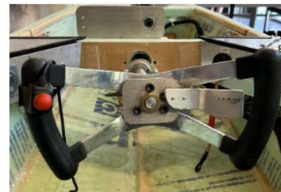
Fig. 7.5- Butterfly steering wheel with custom paddle throttle
