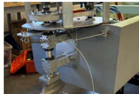
Fig. 7.4- Cables penetrate transom and attached to steering knuckle on lower unit
