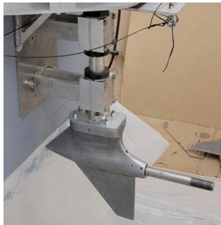
Fig. 6.6a- Sprint output shaft and lower unit, supported by standoffs
