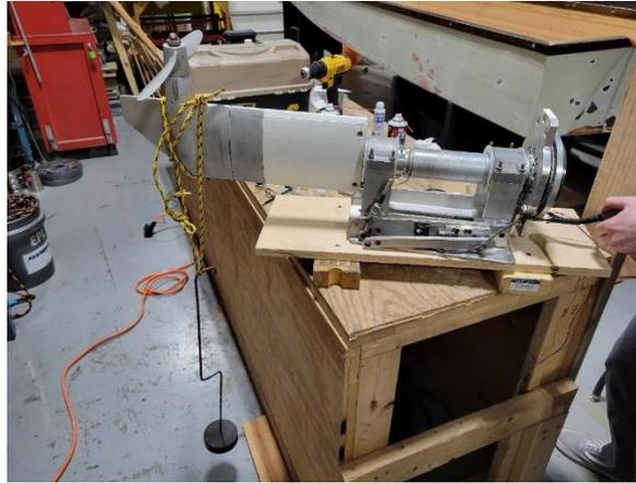
**Fig. 2.17.** Incremented weight test for thrust load cells.
