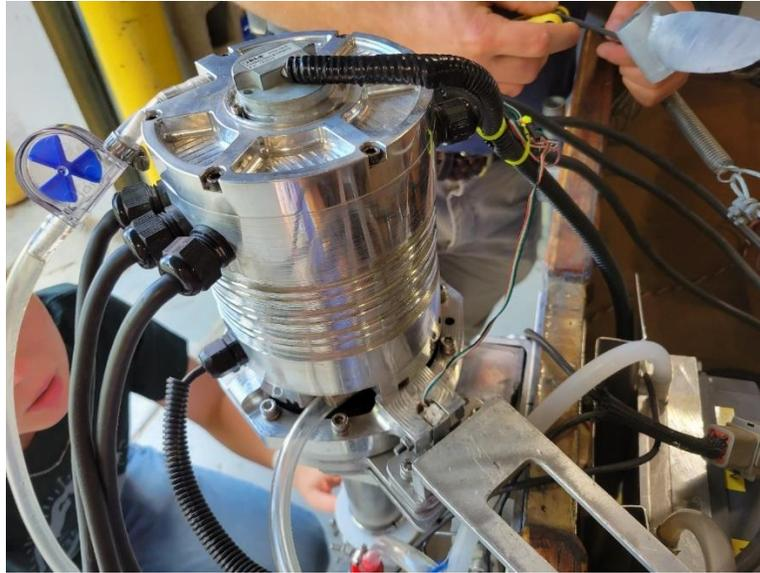
**Fig F.3.** *Original orientation of torque load cell on Solar Splash boat*
