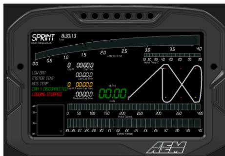
**Fig 2.20.** AEM CD-7L display shown in a simulation from AEMDashDesign software with our design of the screen for the Sprint event.
