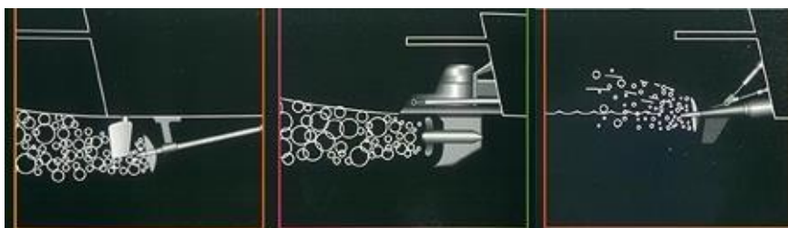
Fig 9: Drag force illustration between inboard, outboard, and surface drive
