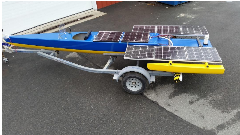
Figure 2: Image of the solar panel layout when mechanically fastened to the boat.
