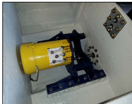
Figure 12: Motor Mount with Motor Embedded in Central Planing Hull
