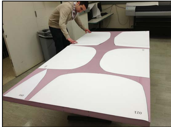
Figure 7: Cross Sections used in Manufacture of 2013 Hull
