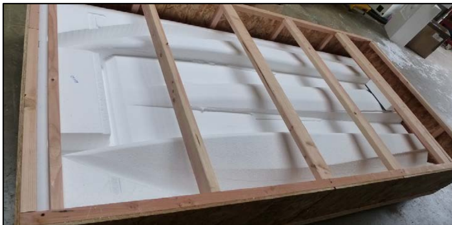
Figure 9: Negative Foam Mold of Hull Design
