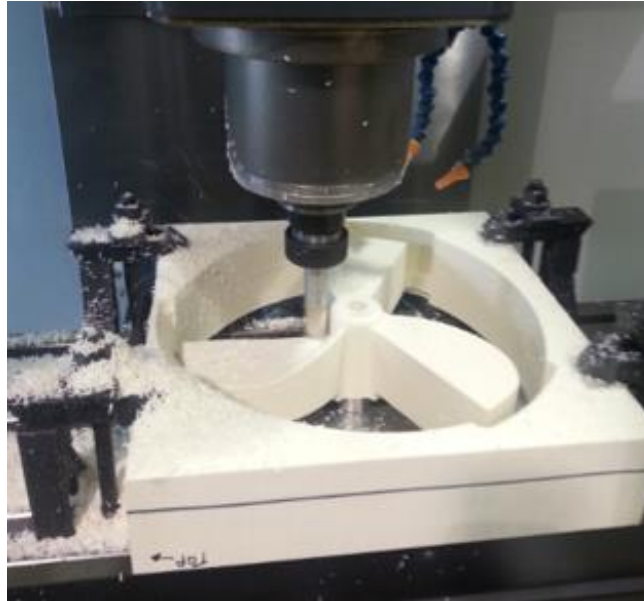
Fig. 20: Butter board Prototype during CNC Mill Machining
