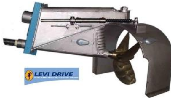
Fig. 12: Fixed Shaft Surface Drive Adapted from Lancing Marine
