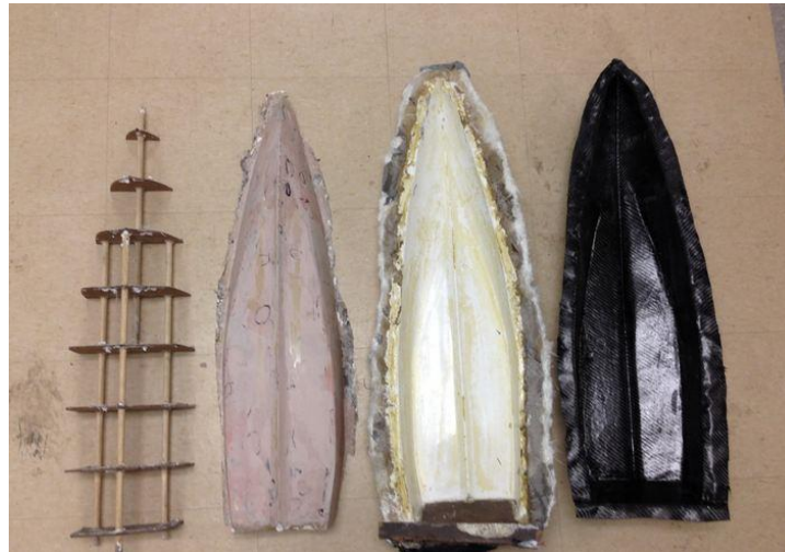
Figure 7: Hull Prototype Fabrication
