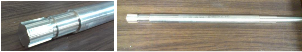
Figure 14: Machined splines on the Propeller Shaft
